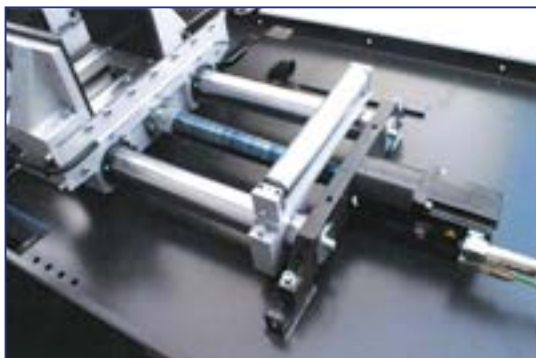
Feed between fixed stops with precise, covered recirculating ball screw and servo drive system
