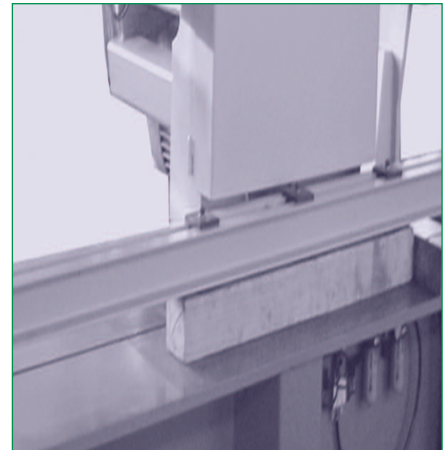
Rip saw with motorized chain drive
