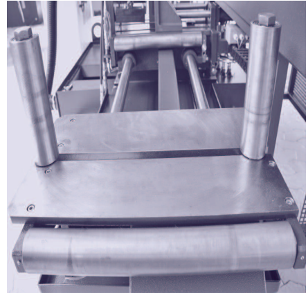
Manual leveling roller on the infeed side
